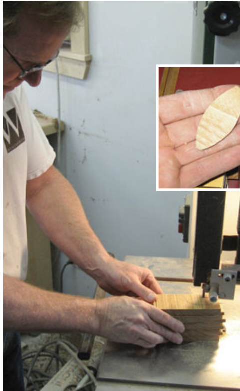
Figure 5. To prevent lateral shifting, a maximum clearance of \frac{1}{4} inch is allowed around the deck's perimeter. The author installed an ipe border in the gap between the parapet and field tiles (above), supported between pedestals with custom-made ipe biscuits (right).
